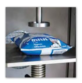
The milk bag is placed on the flat support and a tup, instrumented or not, is released with a predefined energy per the testing standard. A flat surface insert will impact the bag, causing the milk bag to compress. By following this process, quality professionals can verify the impact resistance of the bag. The instrumented tup captures the force of impact onto the bag - allowing users to evaluate the failure force and the energy that is necessary to break the bag.
