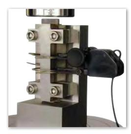
When stiffness is important, using an appropriate testing system is critical. Instron 5900 universal systems are extremely stiff and offer significantly less frame compliance when compared to most other testing systems.
