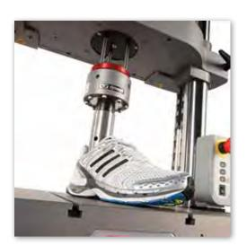
In addition to performing mechanical tests to ASTM F1614, our ElectroPuls® Test Instruments provide flexibility to test other criteria - including the evaluation of energy returned by a shoe during impact, the amount of cushioning provided by different shoe and sole designs, and the long-term fatigue behavior of the shoe.
