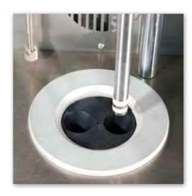
Capillary rheometers allow for an extensive and comprehensive characterization of materials, representing the only off-line way to reproduce processing conditions. Dedicated accessories have been designed for CEAST Capillary Rheometers to measure the pvT of the melt under processing conditions according to ISO 17744. A single capillary rheometer, with its accessories, is capable of providing most of the information needed for an accurate process analysis and simulation.
