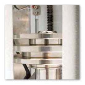
The CEAST MF50 tester performs melt flow tests applying several different load conditions in a single semi-automatic test. Values and sequence of test loads can be selected without changing the instrument configuration. The testing principle is the same as the standard MFR/MVR machines, but allows for higher productivity and comes with a state-of-the-art, user-friendly interface.
