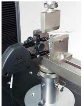
If a direct strain source is being used, we recommend using a deflectometer, a spring-loaded plunger positioned below the specimen. When the specimen starts to flex, the plunger will compress and strain can be measured using an appropriate extensometer. The deflectometer is compatible with certain clip-on extensometers, the Advanced Video Extensometer (AVE 2), as well as the AutoX750 automatic contacting extensometer.
