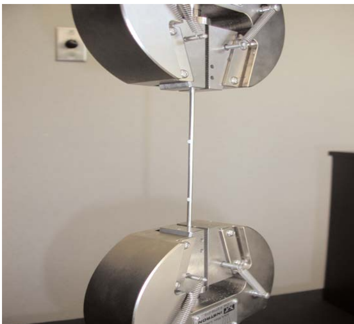
Figure 2: Close-up of the grips and the marking technique recommended for strain measurement with the AVE.
