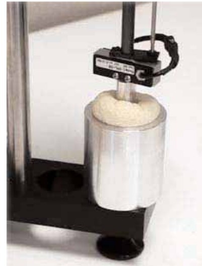
▲ Close-up view of the back extrusion test on pizza dough
