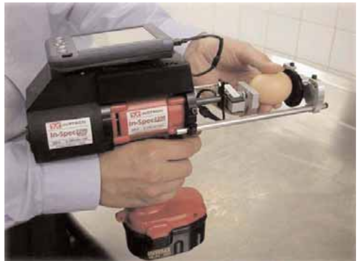
▲ For testing eggs in the field where no AC power is available, there is a handheld version of the In-Spec 2200, which would produce the same information taken in the field.
