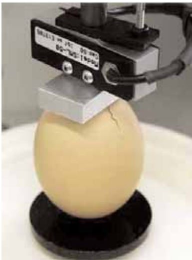
▲ Close-up view of the egg compression test
