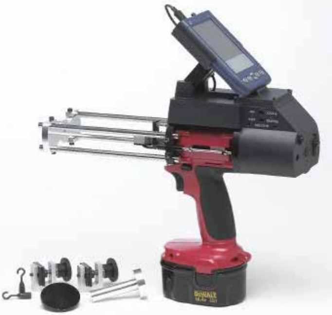
▲ Figure 5: The In-Spec 2200 handheld for applications requiring maximum mobility
