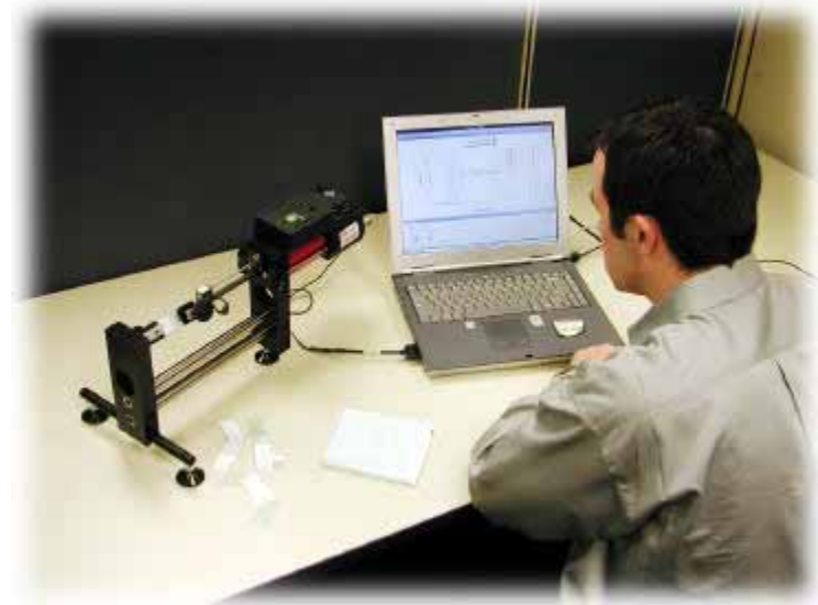
▲ Figure 1: Overall view of the In-Spec 2200 benchtop for ASTM F-88. Configured with laptop and Series IX™ software
