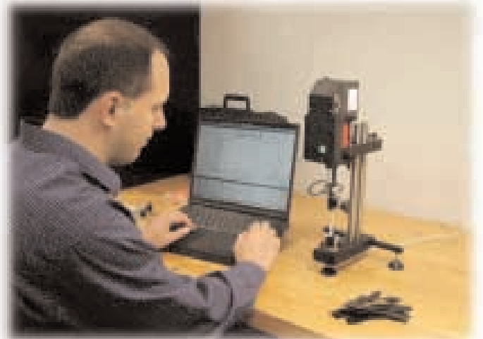
▲ The Bench-Top version of the In-Spec 220 shown with Lap Top/Series IX data acquisition instead of PDA.
