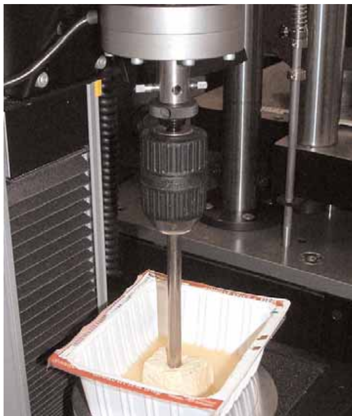
▲ Figure 2: Test configuration for indentation method with tofu sample in container
