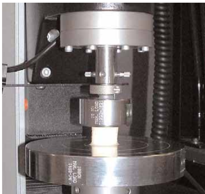
▲ Figure 1: Test configuration for compression method with 1 in diameter tofu specimen
