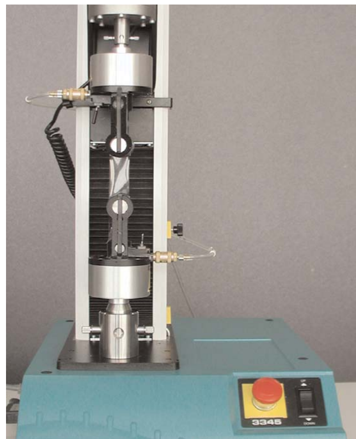
Figure 1: Test configuration for performing tensile test on thin plastic sheeting specimens.
