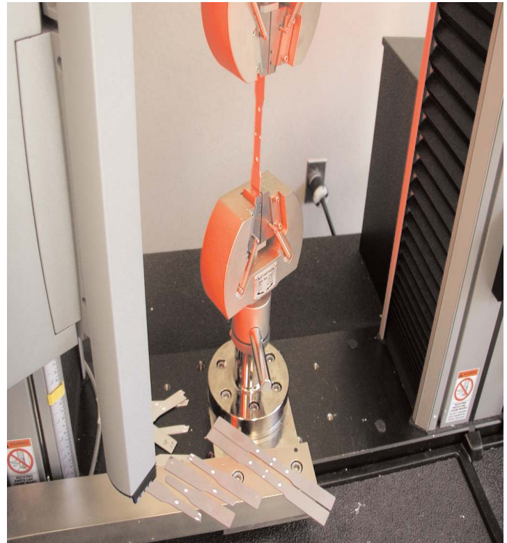
▲ Figure 1: Test configuration for steel specimens tested with the AVE. Specimen is marked with four white dots to measure axial and transverse strain simultaneously.
