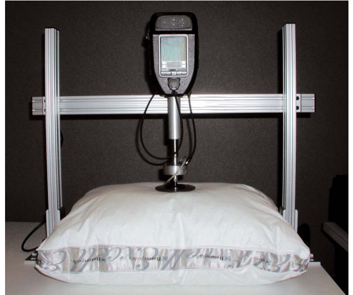
▲ Figure 1: Customized test configuration for evaluating pillow comfort using the In-Spec 2200.
