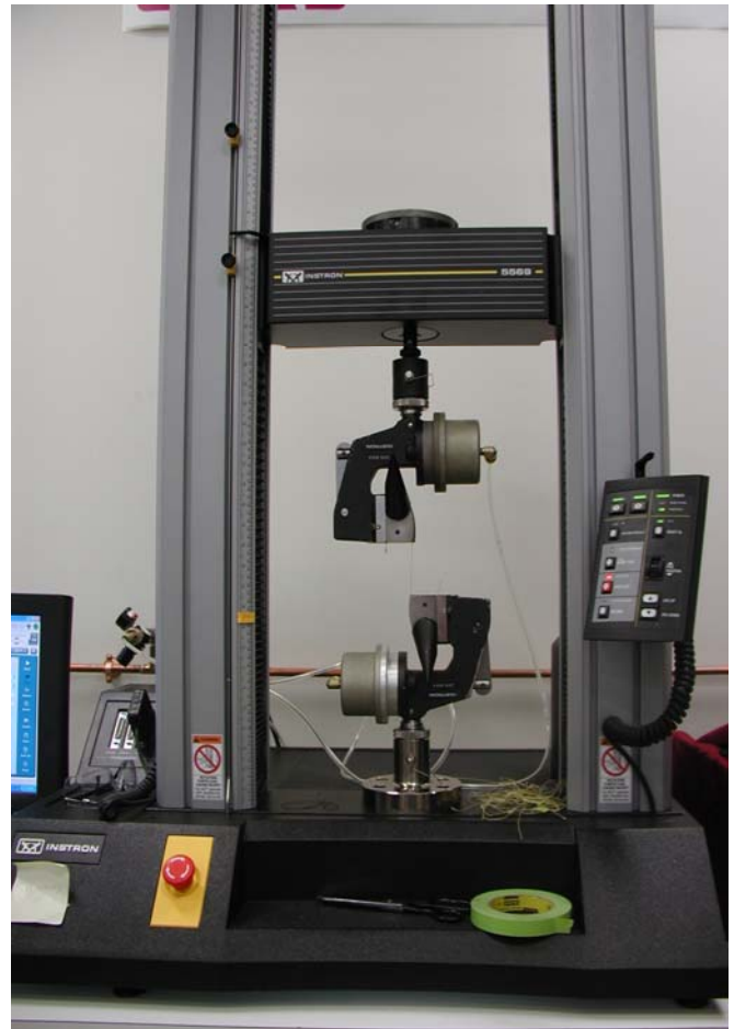
▲ Figure 1: The test configuration, setup on the 5569 dual column testing frame with the 2 kN pneumatic aramid cord and yarn grips, Bluehill® 2 Software and 5 kN static load cell.
