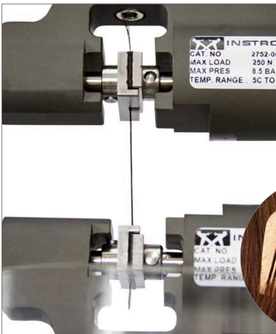
Manufacturers of hair dyes and other hair care products evaluate tensile properties of hair, typically yak hair, before and after treatment with product
