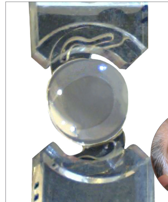
Testing of intraocular lenses to ISO 11979-3 requires a high precision test system with the stability to handle micro-level forces
