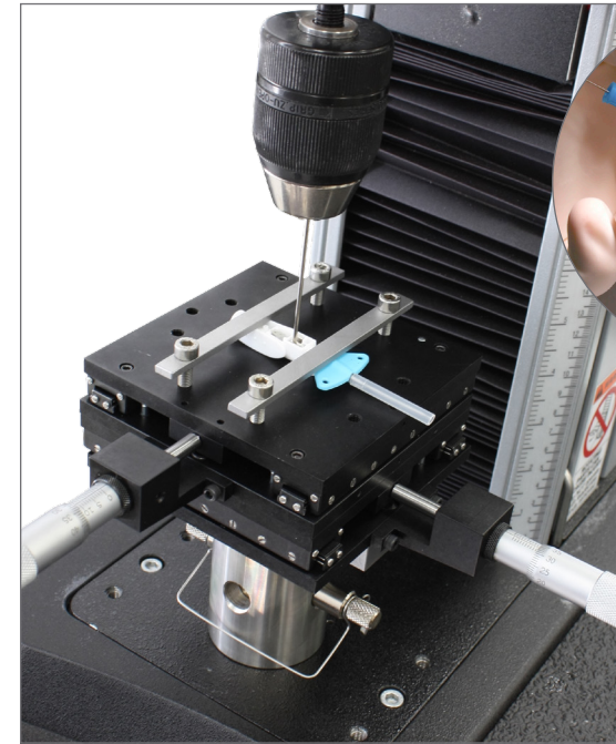
An X-Y Stage helps to perform compression and pull-off tests on catheters & luer locks
