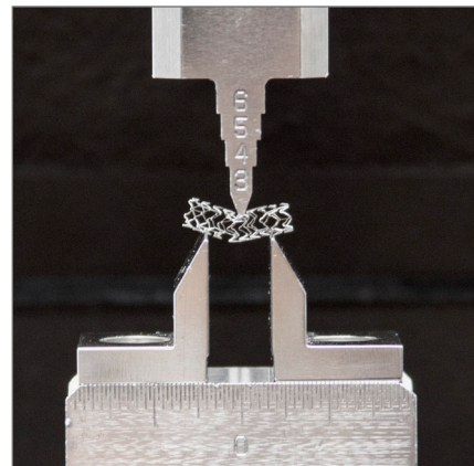
Three-point bending of expandable vascular stents performed to ASTM F2606
