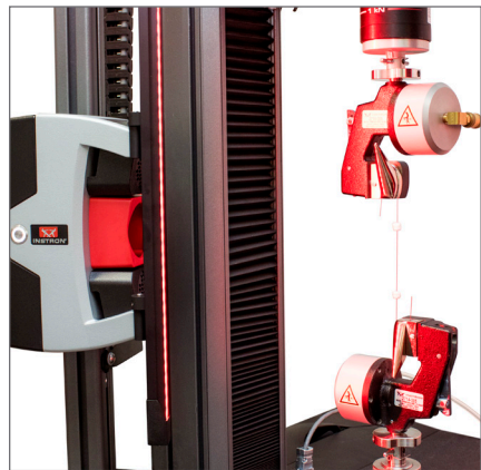
Tensile testing of Nitinol wire to ASTM F2516 using non-contacting strain measurement helps to characterize its use in many implantable devices
