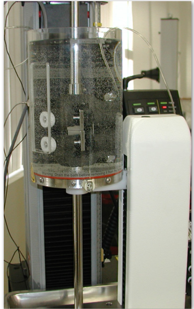
Figure 1: Test configuration for contact lens tensile test using BioPuls submersible pneumatic grips and temperature-controlled bath.
