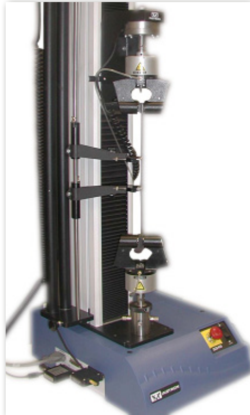
Figure 1: The long travel extensometer was able to accurately measure strain of the tubing specimens through material break.
