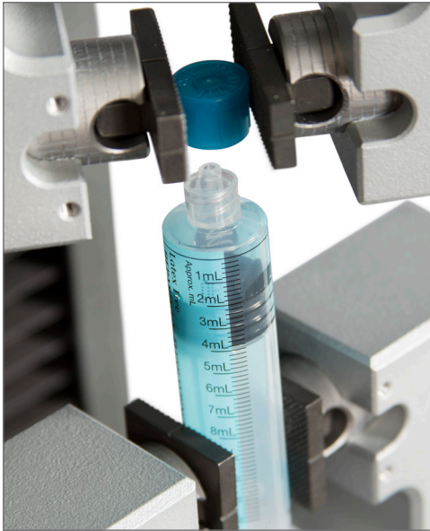
Quantifying torsional properties of syringe caps and luer locks is conducted to ISO 80369-7, ISO 594-1 and ISO 594-2.
