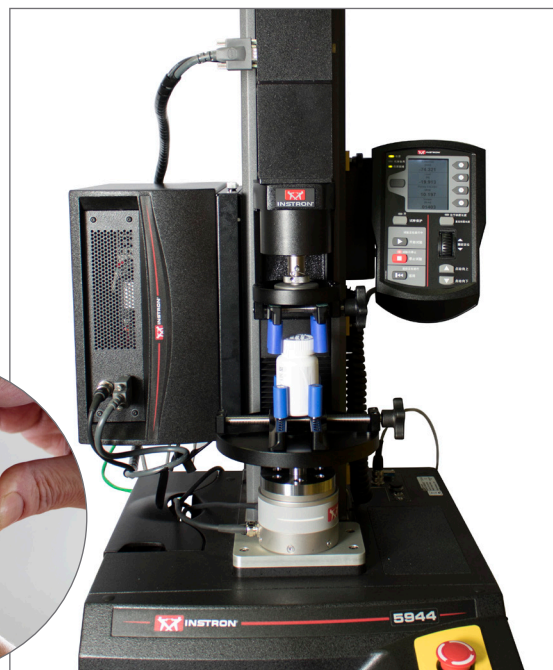
A 5940 single column machine with the torsion add-on applies compressive or tensile loading on a child-proof medicine bottle while simultaneously twisting the cap off.
