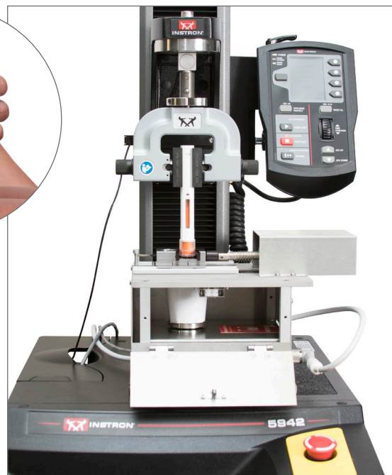
ISO 11608-5 requires needle-based injection systems to be tested for cap removal, activation force and displacement of the injector, injector timing, and measurement of the ejected fluid.
