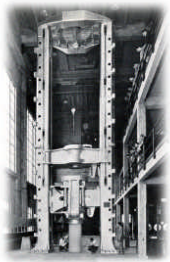
▲ 4,000,000 lbf Southwark-Emery universal testing machine configured for concrete compression testing
