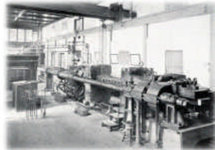
▲ A.H. Emery's world-famous "United States testing machine" was installed in 1879. Capacity: 800,000 lbf (tension); 1,000,000 lbf (compression).
