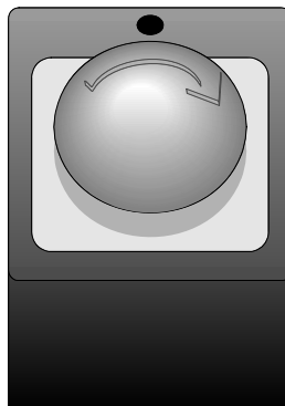
Figure 3-2. Emergency Stop Button
