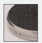
least two and a half times the diameter of the indentation. Tests are to be taken on the top side of the block only.
