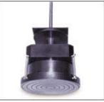
Compression testing can utilize the spherical seating platen to ensure even loading.
