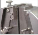
Some grips and fixtures feature specimen stops that allow the specimen to be accurately and repeatably located.
