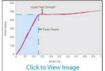
For example, if you run a test in stress control at the onset of yielding, the testing machine will accelerate to maintain the desired stress rate. Incorrectly running in load control causes unwanted acceleration. This prevents the stress from dropping relative to the increase in strain. As a result, the upper yield strength calculation will fail because it can't find the dip in the stress-strain curve (a zero or negative slope).
