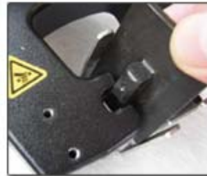
Jaw face changes require no tools or pins
