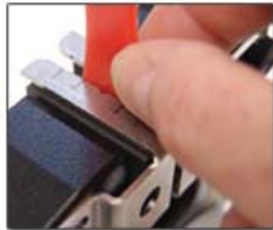
Jaw face shields reduce pinch hazard and feature graduations to aid specimen placement
