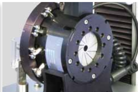
Radial force testing on a coronary stent
