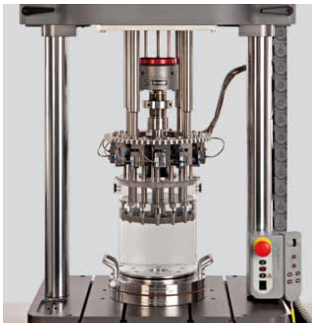
Test fixture on an Instron E3000 testing 12 stents simultaneously in a bath
