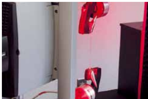
NiTi wire being tensile tested with a video extensometer measuring strain
