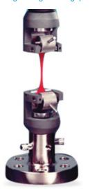
The self-tightening grips are ideal for meeting customers' elastomeric tensile testing requirements at ambient and non-ambient temperatures. These grips have a short effective length so that elongation in a chamber can be maximized.
