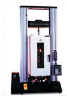
At times, elastomers need to perform at either above or below ambient temperatures. Asphalt and bituminous membranes for flat roofs are being replaced by rubber in many countries. This means the rubber needs to perform over a vast temperature range. Combining the self-tightening grip and an Instron temperature chamber provide customers with a solution that can replicate or get close to 'in the field' conditions.
