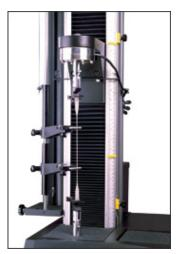
As previously mentioned, elastomers tend to thin as they elongate. This means if the crosshead displacement is used to measure strain then elongation is not only being measured at the gauge length but also outside the gauge length and within the jaw faces.
