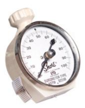
**A.** It's both. A <u>durometer</u> is an instrument used to measure hardness and is typically used on polymeric, elastomeric, and rubber materials. Durometer also refers to the hardness result obtained.
