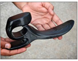
with a heel area, a toe area, and a strong dynamic C-section at the ankle. Each of these act as springs providing elastic energy storage and return during the gait cycle. The properties of the material partnered with the unique structure let the foot mimic biological foot action. Moreover, its comparative low cost means it is potentially accessible to many more people. However, it has taken several years of research and testing for the foot to achieve this performance.
