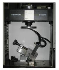
Testing for material characterization, biomechanical evaluations, and overall durability has factored strongly into the development of the foot. Much of the materials characterization testing was performed using Instron® static and dynamic testers at DuPont research laboratories.
