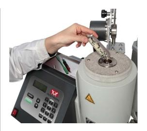
Air bubbles could contribute to inconsistencies in melt flow values. There are many reasons you could be seeing air bubbles in a filament sample. Ultimately, it comes down to keeping the testing and cleaning processes as consistent as possible. There are a few major points to consider.
