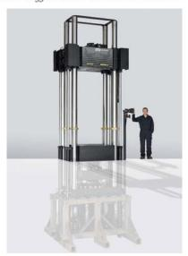
Used to test materials for the San Francisco-Oakland Bay Bridge East Span Seismic Safety Project (SFOBB) - known more simply as the East Span Project - this custom-made testing system has the capacity to test 2,000,000 lbf (9000 kN) in compression and tension.
