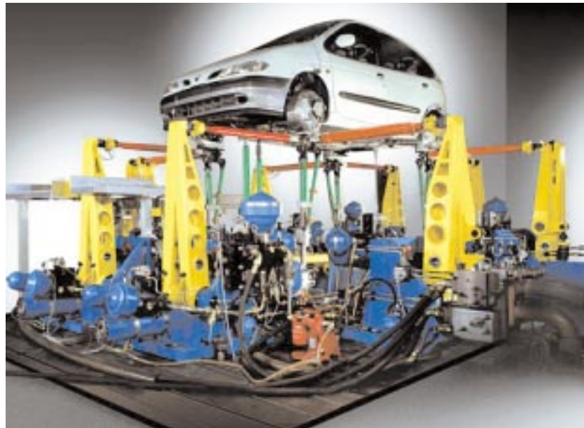
▲ Full vehicle testing system
