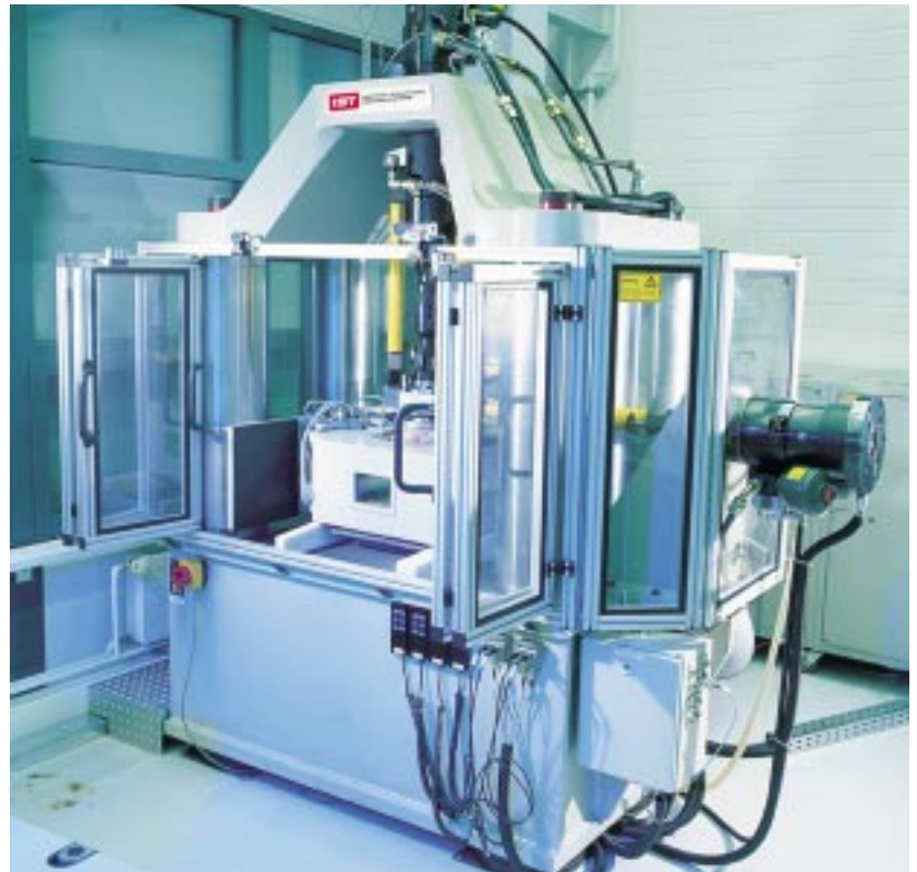
▲ 4-axis test system for evaluation of component properties and endurance testing
