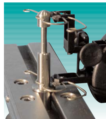
▲ Deflectometer using clip-on extensometer
