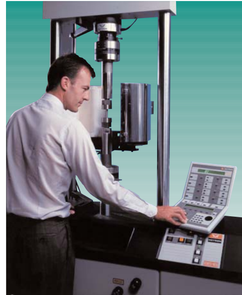
▲ +1000 °C (+1832 °F) pullrods with furnace
