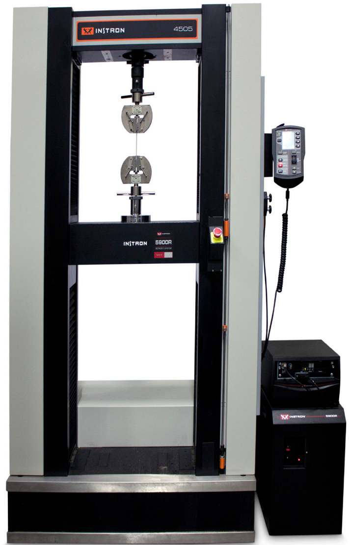
5900 EXTEND Upgrade on Instron 4505 (Power Module Box is not necessary for all system upgrades)
