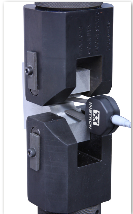
2670-132 COD Gauge fitted to a CT25 specimen
