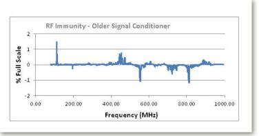
Graphs show the Instron 5900 Signal Conditioner Module's immunity to frequency interference in the frequency band of 80 MHz to 1 GHz (examples include radio, television, or mobile phones). The new Signal Conditioner Module shows a maximum error of 0.025% of full scale load, while the older version shows a maximum error of 1.5% of full scale load - a 60 times improvement.
