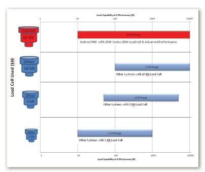
An Instron 5900 system requires less load cells to achieve the same load accuracy measurement range as other systems with load accuracy to 1% of load capacity.
