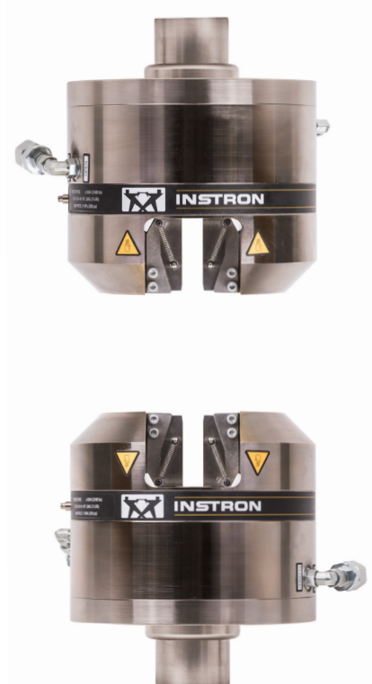
±100 kN (22 kip) universal hydraulic wedge-action grips
