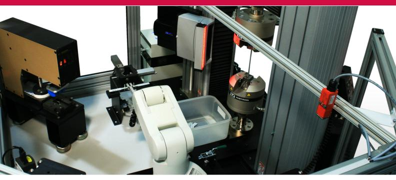
The Instron® Automated Metals Testing Systems enable a new dimension of testing productivity. Available as a complete turnkey solution or installed on an existing Instron testing machine, these systems have been designed to meet ASTM E8, EN 10002-1, ISO 6892, and other metals testing standards, including JIS and DIN.
