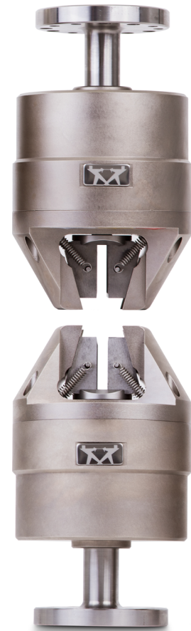
±3 kN, ±25 Nm pneumatic fatigue-rated wedge action grips
