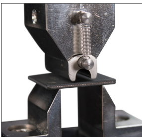
4-Point Bend Test of Electronic Packages
