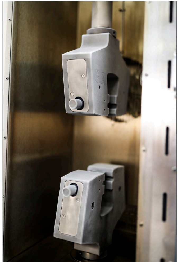
10 kN High Temperature Pneumatic Grips in Chamber
