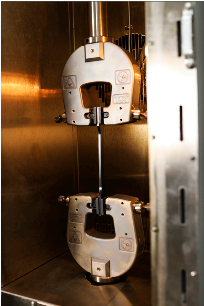
2 kN High Temperature Pneumatic Grips in Chamber
