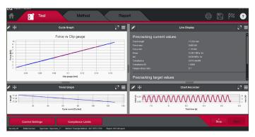
Pre-cracking control is included within the software, allowing data to be automatically collected and included in the validity analysis of the fracture test. Alternatively, pre-cracking data can be entered manually, or generated on another machine running Bluehill Fracture and the test file re-opened providing simple continuity.
