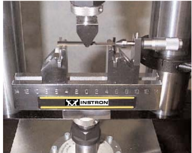
Figure 7. Three-point bend fixture with micrometer for specimen testing
