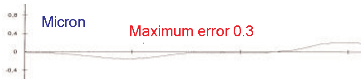
Figure 4. Actuator displacement accuracy over entire stroke
