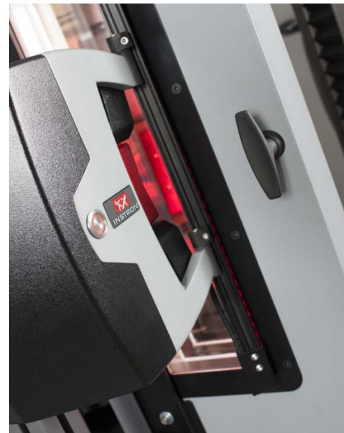
Figure 4 – Non-Contacting Video Extensometer Mounted Outside a Temperature Cabinet
